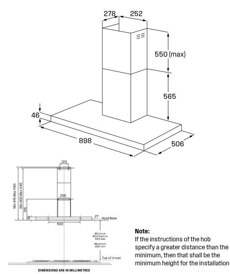
These dimensions are a guide only. All measurements are in millimetres (mm). For complete installation instructions, refer to the manual provided with product.
